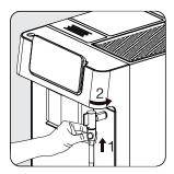
Attach the metal tube back to the nozzle cover. Then push it upward to put the nozzle cover back in its place and turn it to the right to lock it.
