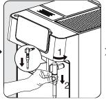
Remove the metal tube by pulling it down. Then remove the nozzle cover by turning it to the left to disassemble the nozzle cover and metal tube.
