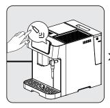
Press steam nozzle icon and wait for steam nozzle to be ready. While steam nozzle is pre-heating, the indicator lights will flash.
